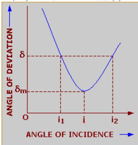
The angle of deviation of a ray of light in passing through a prism not only depends upon its material but also upon the angle of incidence. The above figure (2) shows the nature of variation of the angle of deviation with the angle of incidence. It is clear that an angle of deviation has the minimum value ' $\delta_m$ ' for only one value of the angle of incidence. The minimum value of the angle of deviation when a ray of light passes through a prism is called the angle of minimum deviation.
