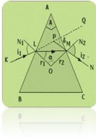
Figure (4) shows a prism having a very small refracting  $\angle A$ . a ray KL is incident on the face AB such that the angle of incidence 'i' is very small. Accordingly, the angle of refraction 'r' will also be very small. Also angles 'r<sub>2</sub>' and 'i<sub>2</sub>' must also be very small. If ' $\mu$ ' be the refractive index of the material of the prism, then
