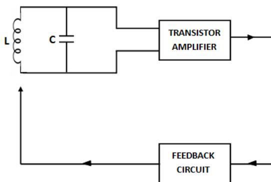
It's essential components are (i) tank circuit, ii) amplifier and (iii) feedback circuit.
