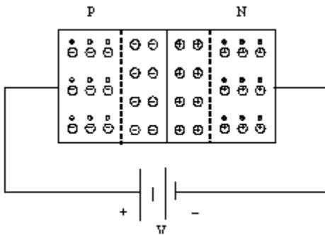
When the PN junction is reverse electrons in the N region and holes in the P region are attracted away from the junction N-side and negative terminal to the P-side, so that the applied potential. Because of this, the number of negative ions in the P-region and positive ions in the N-region increases. Hence the depletion region becomes wider and the potential barrier is increased.
