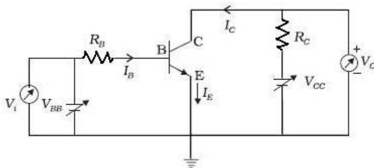
We shall try to understand the operation of the transistor as a switch by analyzing the behavior of the base-biased transistor in CE configuration as shown in Fig.
