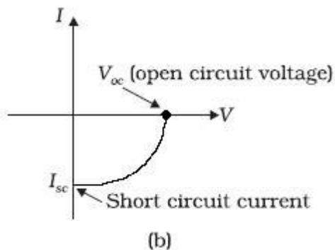
Note that the I – V characteristics of solar cell is drawn in the fourth quadrant of the coordinate axes. This is because a solar cell does not draw current but supplies the same to the load. Semiconductors with band gap close to  $1.5\ \text{eV}$  are ideal materials for solar cell fabrication. Solar cells are made with
