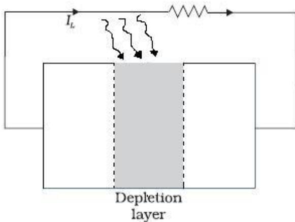
(i) generation of e-h pairs due to light (with  $h\nu > E_g$ ) close to the junction;
