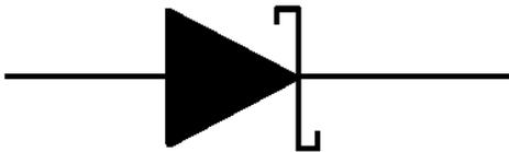
Zener diode is fabricated by heavily doping both p-, and n- sides of the junction. Due to this, depletion region formed is very thin ( $<10^{-6}$  m) and the electric field of the junction is extremely high ( $\sim 5 \times 10^6$  V/m) even for a small reverse bias voltage of about 5V. The I-V characteristics of a Zener diode is shown in Fig
