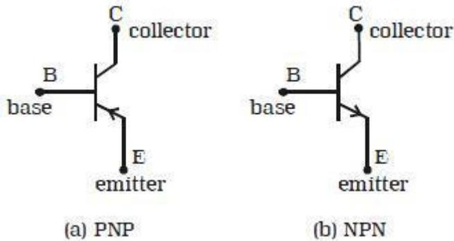
The arrow on the emitter lead pointing towards the base represents a PNP transistor. When the emitter-base junction of a PNP transistor is forward biased, the direction of the conventional current flow is from emitter to base.
