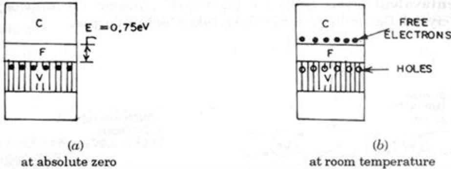
The electrons in an intrinsic semiconductor, which move in to the conduction band at high temperatures are called as intrinsic carriers. In the valence band, a vacancy is created at the place where the electron was present, before it had moved in to the conduction band. This vacancy is called hole.
