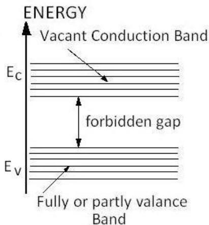
valence band, the electrons from the valence band can move into the conduction band
