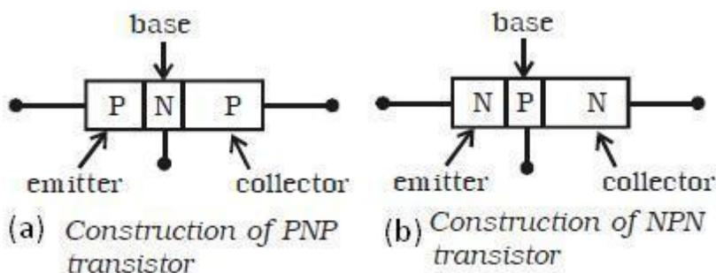
For a transistor to work, the biasing to be given are as follows :
