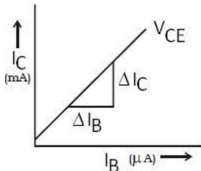
The current gain is defined as the ratio of a small change in the collector current to the corresponding change in the base current at a constant  $V_{CE}$ . current gain,  $\beta$
